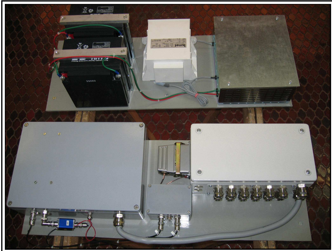
cabin equipment (power supply, electronic box, transmitter/receiver coil, connection box)
